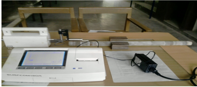
Figure 4: Surface Roughness Tester: - Tokyo Seimitsu Surfcom 130A
