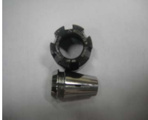
Figure 2.a. Rego-Fix microbore collet &amp; chuck
